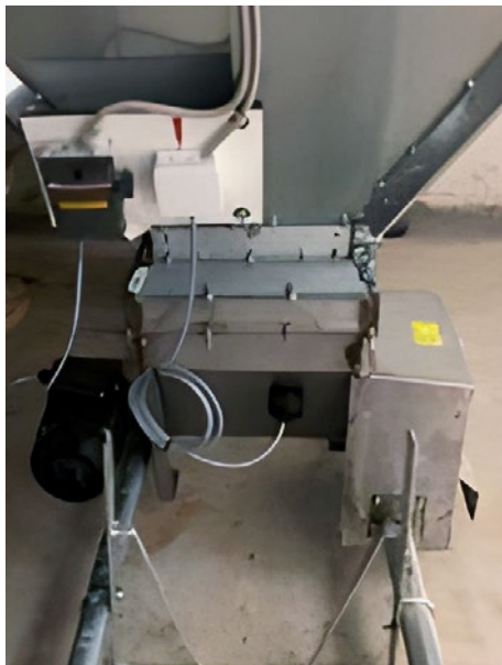
Hopper installed on indoor silo.
